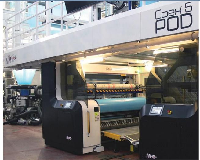
Macchi's POD 5-layer coextrusion line.
