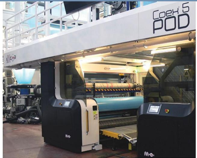
Macchi's POD 5-layer coextrusion line.
