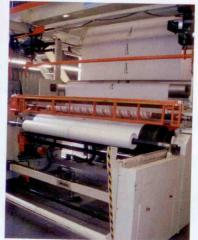
The new line, which has 65-75-65 mm extruders with 400 mm die lip, is equipped with an automatic width control system, 1+3 component gravimetric blending/feeding system, touchscreen SCADA-based control panel and on-line printing, making it user-friendly and allowing for quick changes with minimum wastage, says the machinery supplier
